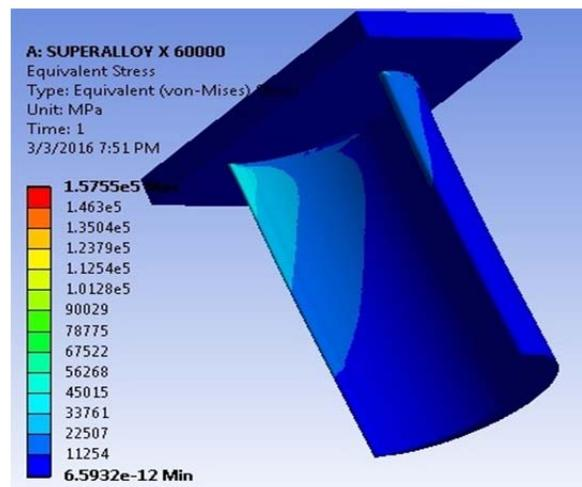
Deformation on Super Alloy X Blade at 60000 RPM
