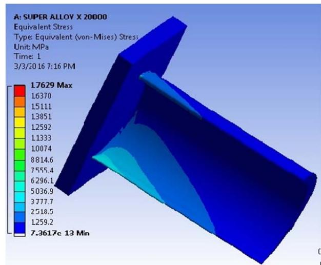
Deformation on Super Alloy X Blade at 20000 RPM
