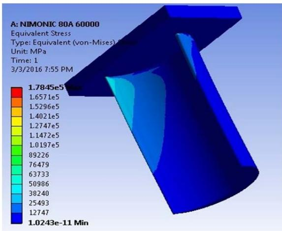
Deformation on Nimonic 80A Blade at 60000 RPM
