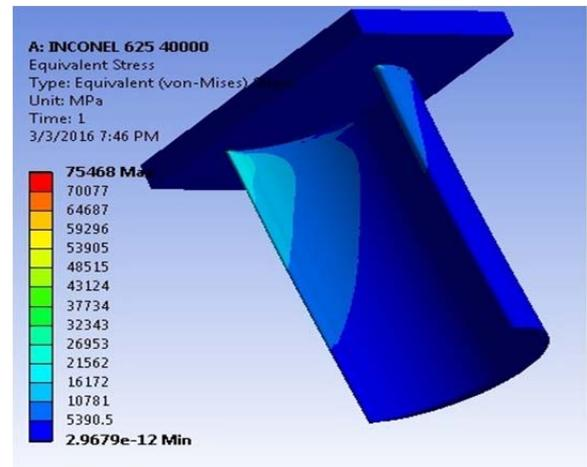
Deformation on Inconel 625 Blade at 40000 RPM
