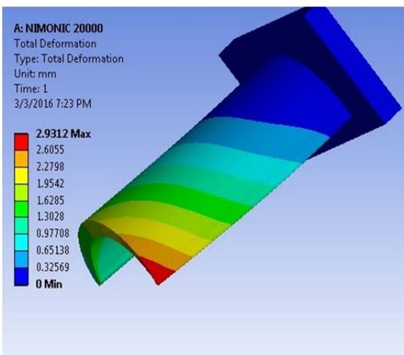
Stress on Super Alloy X Blade at 40000 RPM
