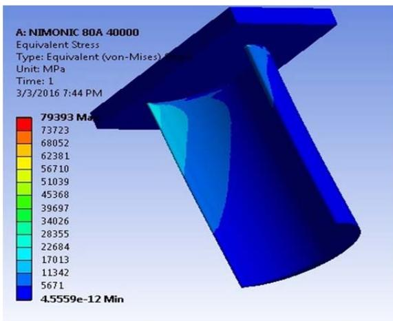
Deformation on Nimonic 80A Blade at 40000 RPM
